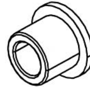
#35 \varnothing 7/8" Pulley Bushing (Qty 6)
